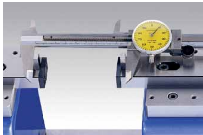
▲ Checking of calipers using 54-196-006
