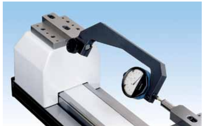
▲ Checking of dial indicators and dial comparators up to 2"/50mm range using dial indicator holder (54-197-015)
