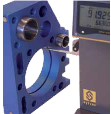
Internal measurements with ruby ball probe Ø3mm, 54-930-211
