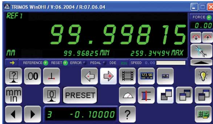
▲ Computer assisted display using Trimos Win DHI XP software (Digital Display)
