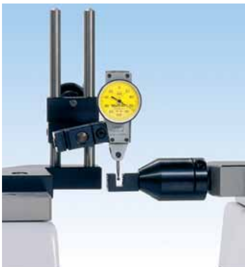
▲ Checking of lever (test) dial indicators using 54-197-115
