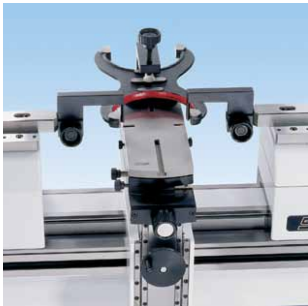
▲ Checking of snap gages with range from .473 to 6"/12 to 150mm using table (54-197-011), snap gage holder (54-197-014) & L-probes (54-197-162)
