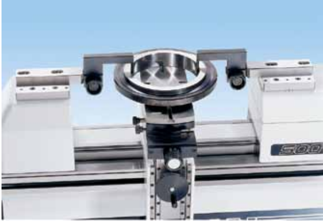
▲ Checking of ring gages from dia. .473"(12mm) to 10"(250mm) using table (54-197-011), clamps (54-197-142) & L-probes (54-197-162)
