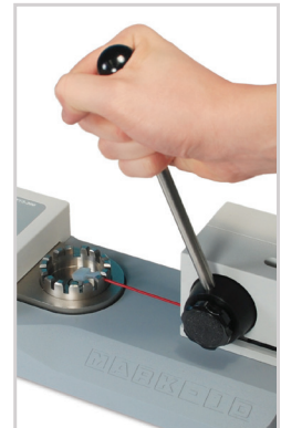
^ Ergonomic lever easily applies force and releases the sample.
