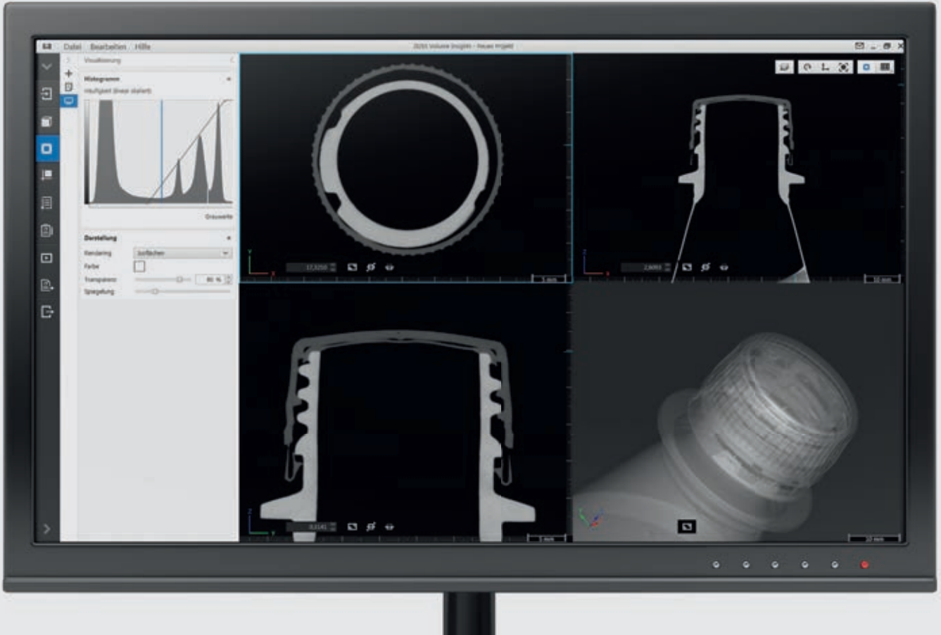
The CT data display using ZEISS NEO insights software shows if the seal is properly positioned on the bottle.
