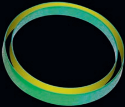
The nominal data of the product (yellow), the current tool shape (green) and the areas which must be corrected (white) in one display
