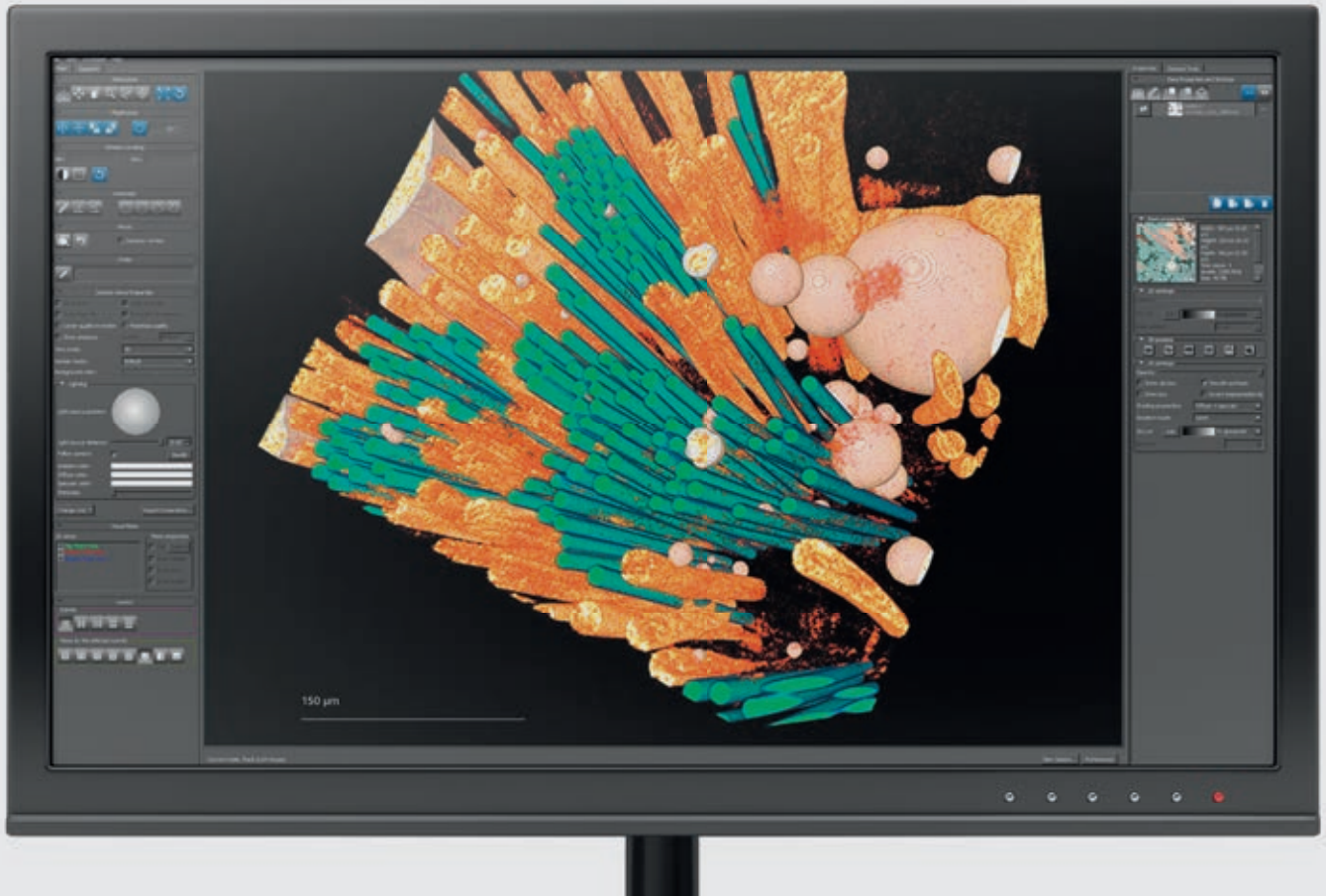
A segmented 3D rendering of the compound material shows glass fibers (green), polypropylene fibers (orange), and voids (white). The sub-micron 3D data shows that the distribution of glass fibers through the matrix does not appear uniform, which may have an effect on material property. The occurrence of air voids with a variety of size could also affect material strength. Courtesy of Professor Abbas S. Milani, University of British Columbia.
