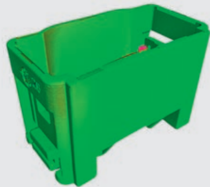
Detection of a material overhang (red) in ZEISS CALYPSO CT
