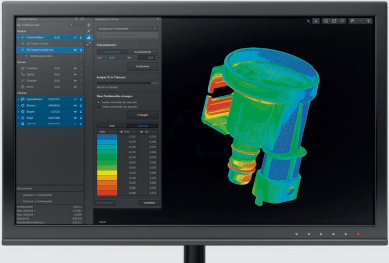
The color-coded display in ZEISS REVERSE ENGINEERING shows you at a glance where and by how much the component diverges from the nominal data. A shift into the blue spectrum indicates undersize whereas a shift into the red spectrum indicates oversize.
