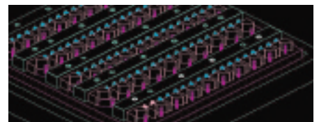
■ A multi-station fixture with spring-loaded Vs to secure different diameters (shown in dwg).
