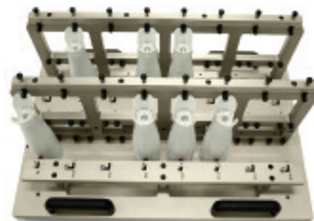
■ Fixture to hold up to 16 parts vertically at one time.
