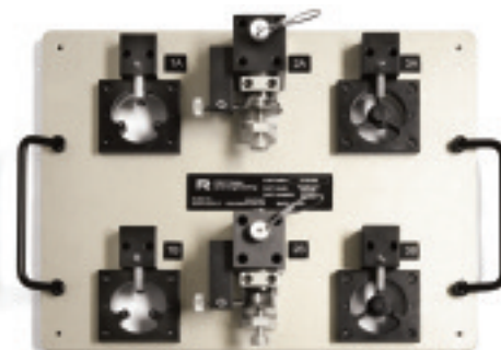
■ Fixture for holding a part in 3 different orientations.
