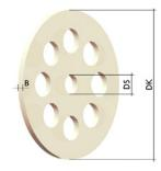
The ball stylus discs from ZEISS are distinguished by a low weight and excellent accuracy of form, even with large diameters. They are made of aluminium oxide ceramic. The roundness is better than 2  $\mu$ m. They can be securely mounted on stylus systems with an M5 thread by means of the holder without any problems. The receiver side of the clamping holder remains on the stylus extension.
