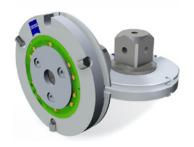
These adapter plates for VAST<sup>®</sup> are provided with an ID-chip for reliable identification by the ZEISS CMM. Furthermore, they are equipped with a 20 mm cube that has already been aligned. Five M5 connections can accommodate styli and extensions. The reference adapter plate is marked with a red ring.
