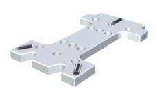
The base mounting plate is mounted directly in the measuring range of your coordinate measuring machine. The appropriate interchangeable pallets can be quickly and easily mounted by hand on the statically defined support with three rollers and with repeated accuracy.
