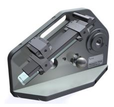
The Multisensor-Check is a procedure for the standardised checking of coordinate measuring machines (CMMs) with tactile/optical sensors. The universal calibration artifact is supplied with the associated control and analysis software. The Multisensor-Check can be used to check coordinate measuring machines in accordance with DIN EN ISO 10360-2 and VDI/VDE 2617 Sheet 6.1:
