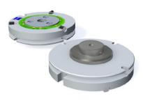
These adapter plates for VAST<sup>®</sup> are provided with an ID-chip for reliable identification by the ZEISS CMM. In addition to this, they are equipped with an M5 holder. An M5 stylus or an extension with a diameter of 20 mm can be attached to this in a vertical direction. As a result of their flat design, they are ideal for use with the Z measuring range.
