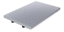
This 300 x 200 grid pallet with changer system has a 25 mm M6 hole line spacing. As a result, user-defined workpiece holding fixtures with bracket clamping systems or other elements can be assembled. You will find suitable clamping material in our clamping kit.
