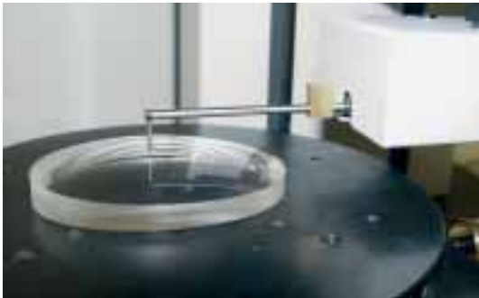
Example application: asphere measurement on a lens
