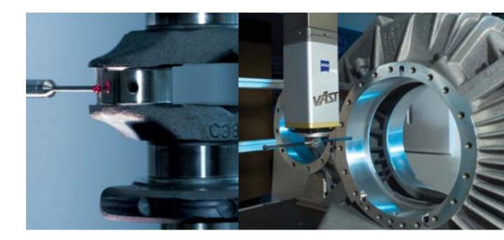
When PRSIMO was designed, the interaction of its component was optimized to provide reliable speed and precision for a variety of measuring needs. Curves, freeform surfaces or gears - the VAST Universal Probe Head for multipoint or single-point measuring flexibly adapts to each measuring task. The integrated Navigator technology ensures higher productivity with more accuracy. PRISMO delivers peak performance to the production environment. Productivity you can rely on.
