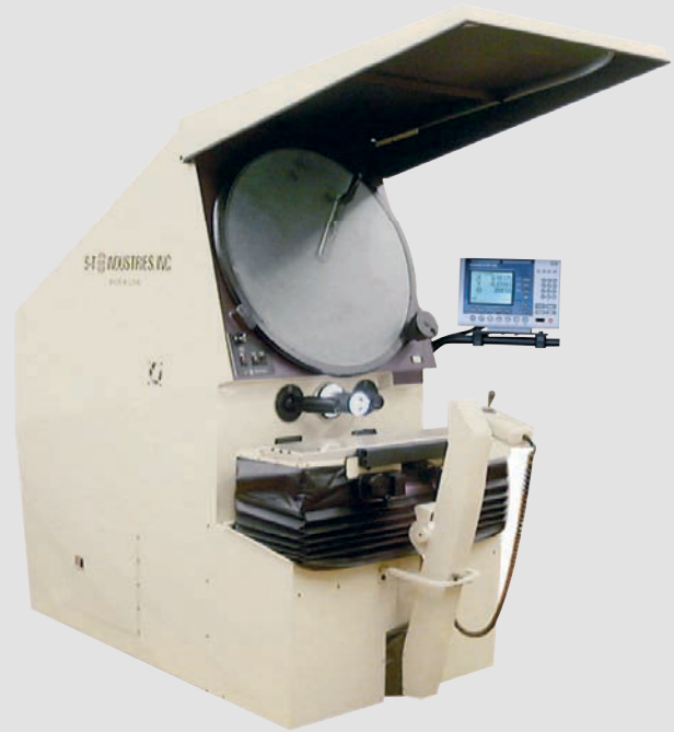
Above: Actual photo of the same 2600 Series 30" Comparator after being remanufactured at S-T Industries, ready to ship back to the customer.
