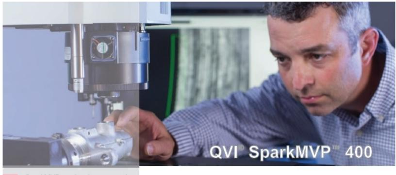
SparkMVP 400 is a large capacity dimensional measuring system designed for measurement of small parts or features. An optional extended Z-axis provides added range for larger parts.
