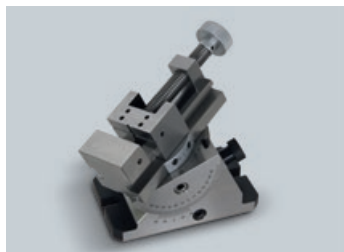
Precision angle vise Tip range \pm 70^\circ , rotation range 0^\circ , ideally suited for the precision positioning table Cat. no. 626108-9010-000
