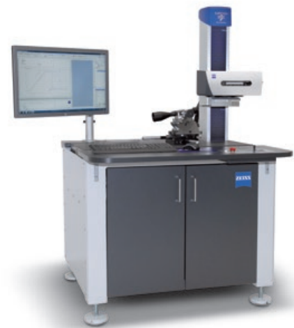
FX version: a compact and active vibration-damping base
