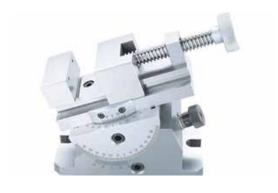
Bench vise can rotate and swivel in 2 axis with a jaw width of 70 mm and a span width of 80 mm. The tilting area is  $\pm$  45°. The rotary area is 360°. The rotatable bench vise is made of steel and delivered with the required fastening material. The bench vise can be mounted directly to the Surfcom.
