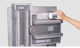
The variety of the fields of application is completed by a broad range of practical accessories. Thus almost every measuring task is possible, be it the Handysurf in any position or even with an interface to the ZEISS measuring software Calypso.
