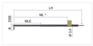
\* Note: This is your desired depth of immersion and not the actual position of the counterweight.
