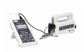
Model combination with small genuine type 50mm tracing driver of S130A. Small tracing driver, available skidless measurement and waviness measurement. Achieve class highest straightness accuracy 3µm/50mm Easy levelling adjustment by tilting support function.
