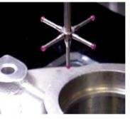
Contact sensors can reach areas inaccessible to video, allowing more measurements of a part in a single setup. QVI<sup>e</sup> multisensor systems can combine video and touch probe measurements in a part routine, saving time and minimizing part handling.
