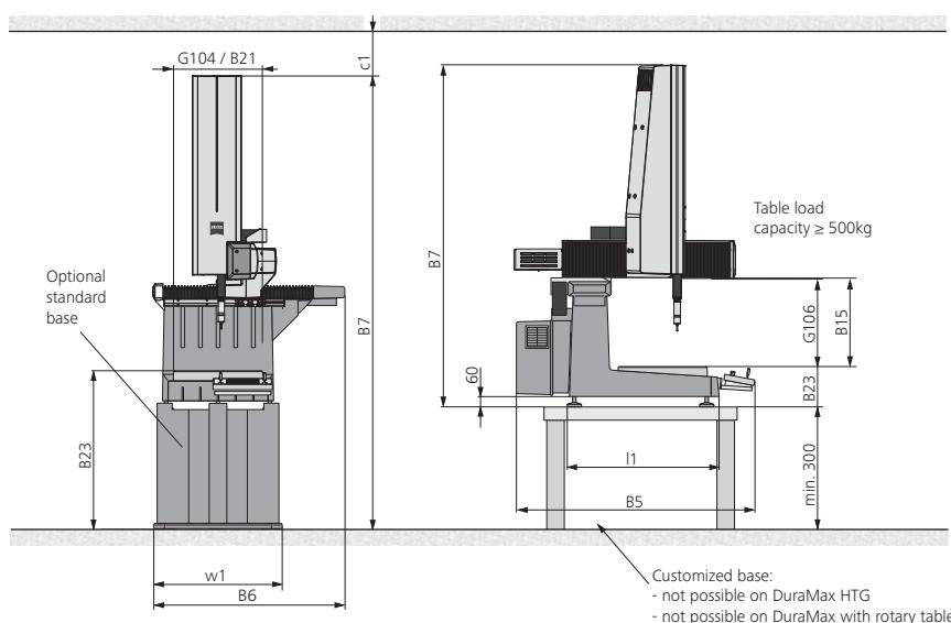
Note: the given dimensions and weights are approximate values. Dimensions in mm. Subject to change. Dimensioning based on DIN 4000-167:2009. If customers use their own base, then a locking mechanism must be used to prevent the DuraMax from slipping! If the ZEISS base is used, a locking mechanism is already integrated.
